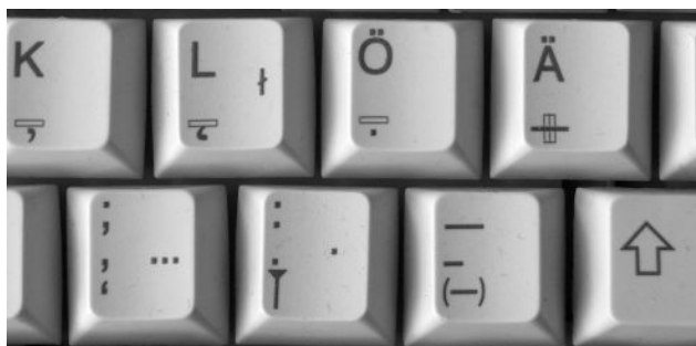
Fig. 1: Detail of a German standard keyboard according to DIN 2137-1:2012-06, showing some of the ISO/IEC 9995-7 and 9995-10 symbols proposed here as Unicode characters.
