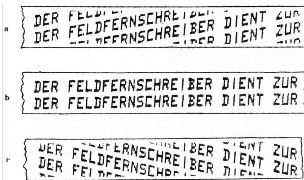
Figure 6 Printed text for speed of the own motor-generator that is too high (a), correct (b), and too low (c)
