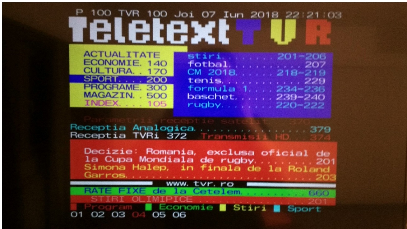
Figure 13. A present-day example of digital teletext in Romania, using block semigraphics from the teletext character set. (Ricardo Bánffy)
