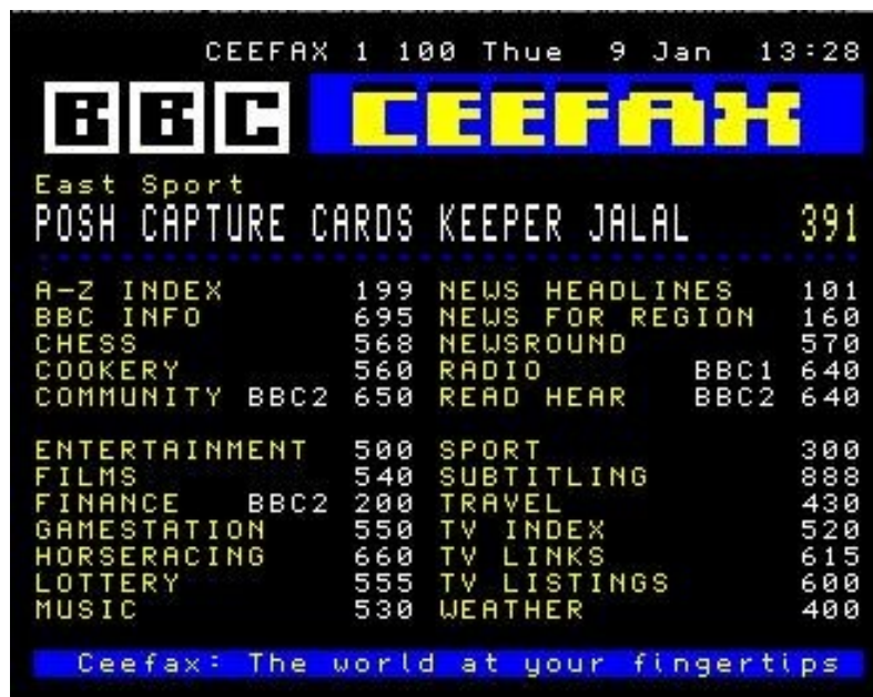
Figure 11. Screen shot from CeeFax, the world’s first teletext information service. Note the use of foreground and background colors, double-height text, and semigraphics.
