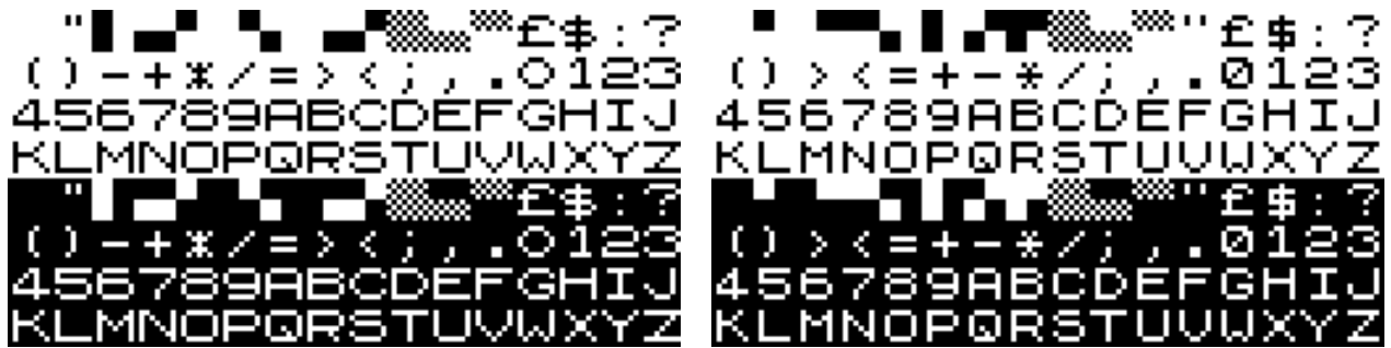
Figure 5. Sinclair ZX80 (left) and ZX81 (right) character dumps. (Wikipedia, CCO 1.0)
