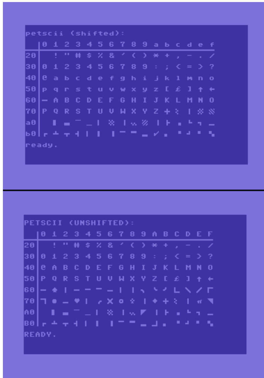
Figure 7. PETSCII as displayed on the Commodore 64. Other Commodore models used slightly different versions of this set. (Wikipedia)
