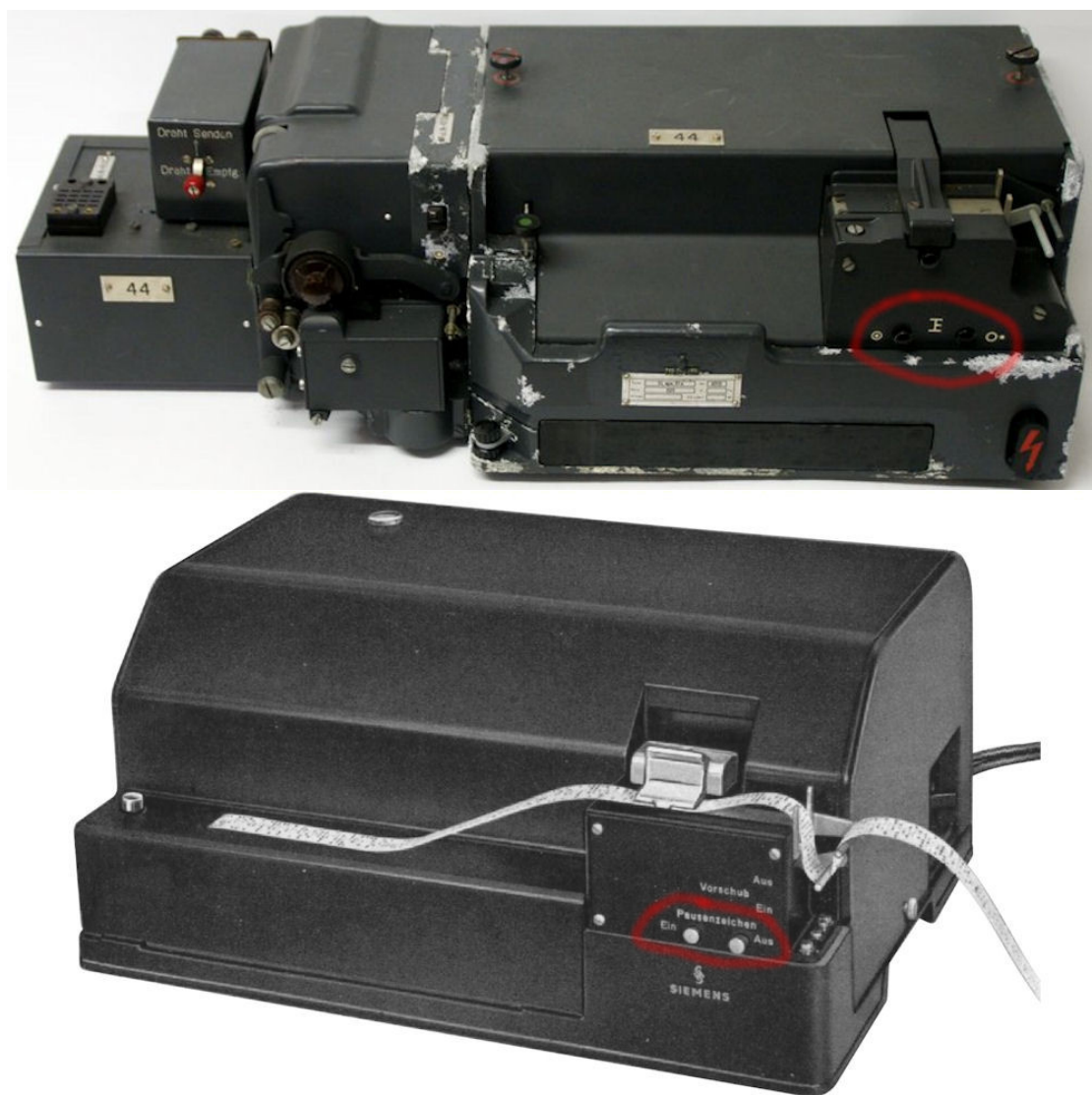
Figure 2: Samples of Hellschreiber teletypers with pause keys
