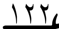
Figure 3: rendering of character sequence (U+202E, U+0600, U+0661, U+0661, U+0662) by Pango 1.14.4 using the SIL font Scheherazade
