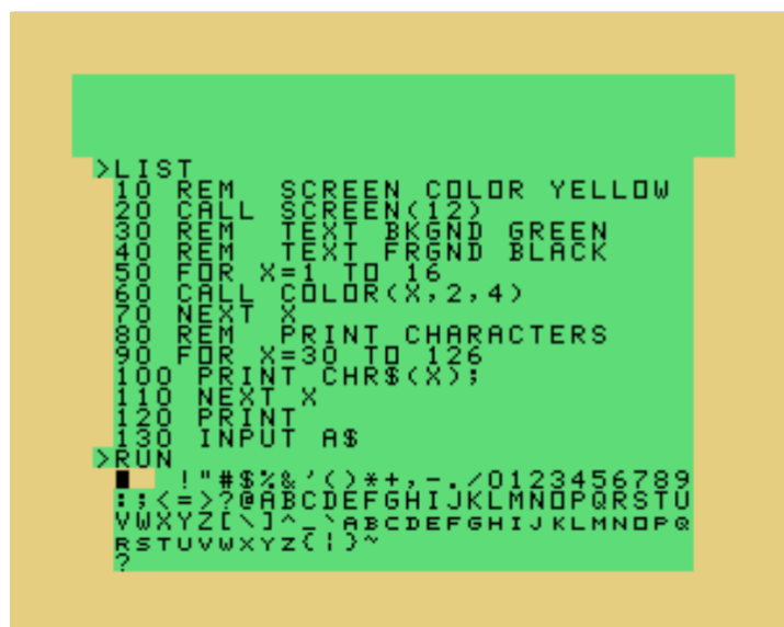
Figure 5. TI-99/4A character dump, generated by Rebecca Bettencourt using a JavaScript-based emulator, showing BORDER-COLOURED FULL BLOCK (the yellow square under the U of RUN).
