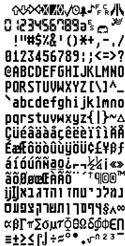
Figure 4. Atari ST glyphs, 8 pixels high (left) and 16 pixels high (right). Note 7-segment styled digits at 0x10 through 0x19 (proposed), and Atari logo at 0x0E–0x0F and J.R. “Bob” Dobbs image at 0x1C–0x1F (not proposed; see Section 8). (Wikipedia, CCO 1.0)
