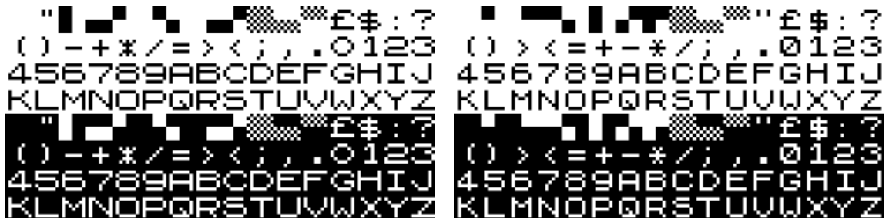
Figure 3. Sinclair ZX80 (left) and ZX81 (right) character dumps. (Wikipedia, CCO 1.0)
